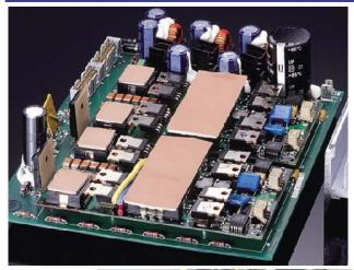
TIF<sup>TM</sup>200-01U Series thermally conductive interface materials are applied to fill the air gaps between the heating elements and the heat dissipation fins or the metal base.
